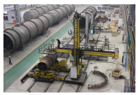
Welding center in pressure vessel industry
